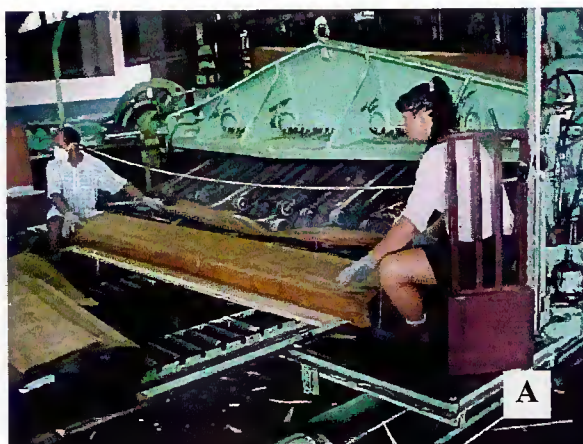
Figura 36. Faqueadeira vertical (A) e horizontal (B)
